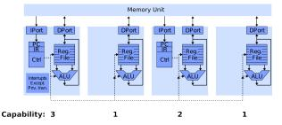
Fig. 4. Example of a ParaNut instantiation with cores of different capabilities
