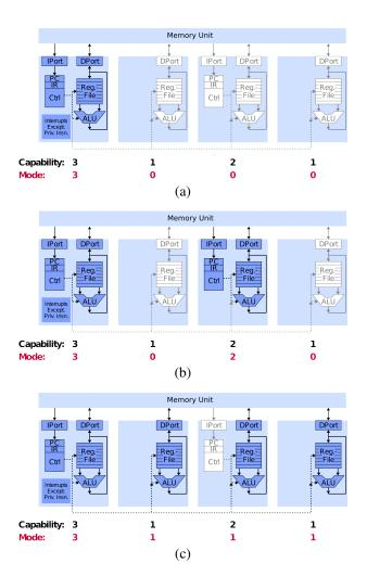
Fig. 5. ParaNut of Figure 4 running a) single-threaded code, b) two independent threads, and c) 4-way vectorized SIMD code
