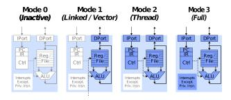
Fig. 3. Modes of a ParaNut core
