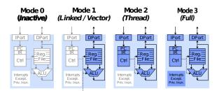
Fig. 5: Modes of a ParaNut core
