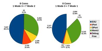
Fig. 10: Distribution of slices over main components of a *ParaNut* processor using 8 cores with different capabilities
