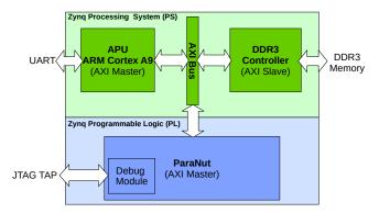
Fig. 8: Block diagram of the ParaNut/RISC-V system
