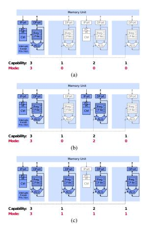
Fig. 7: *ParaNut* of Figure 6 running (a) single-threaded code, (b) two independent threads, and (c) 4-way vectorized SIMD code
