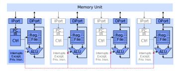
Fig. 2: ParaNut processor operating in linked mode
