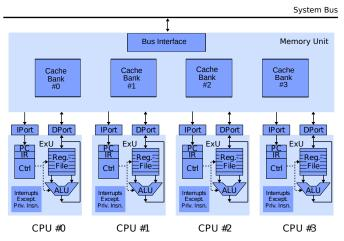
Fig. 1: Block diagram of a ParaNut with 4 (full-featured) cores
